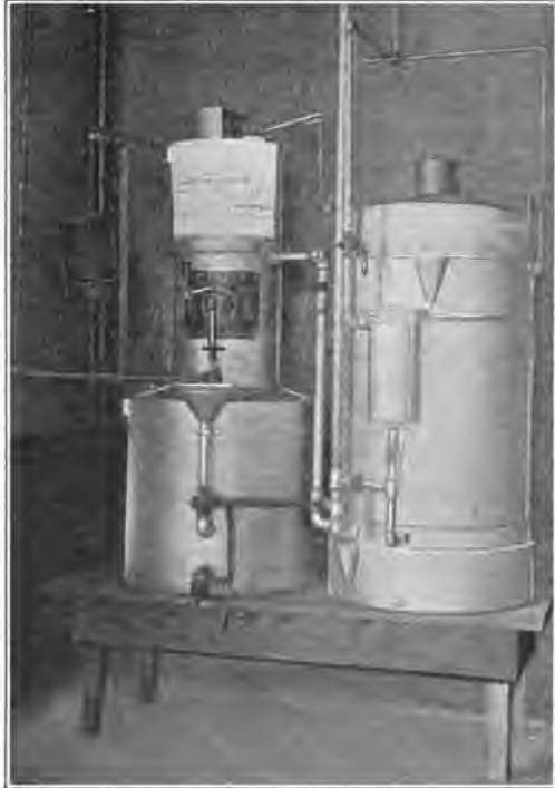
Fig. 315. A 35-light acetylene generator.
