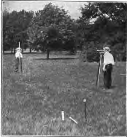
Fig. 50. Taking levels in making a survey.
