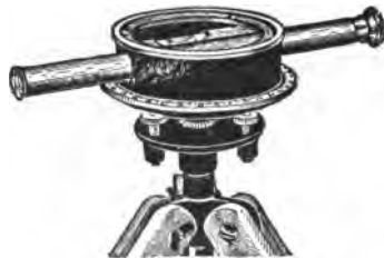
Fig. 34. An inexpensive farm level with horizontal circle for turning off angles.
