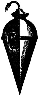
Fig. 30. A plumb- bob with line attach- ed
