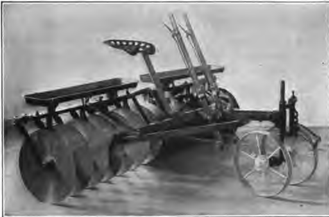
Fig. 123. A full-blade, two-lever disk harrow with tongue truck.
