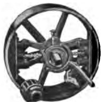
Fig. 238. One form of clutch. The wooden shoes are forced outward against the rim of the wheel, engaging it by friction.
