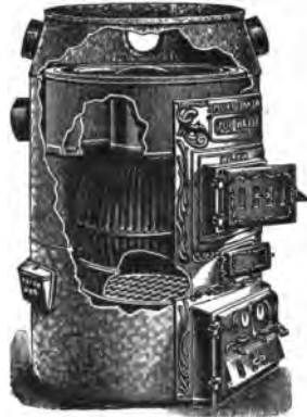
Fig. 319. A typical warm-air furnace.
