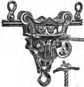
Fig. 173. A hay carrier on a steel track.
