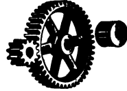
Fig. 207. Spur gearing. The pinion or small gear to the right is "shrouded."
