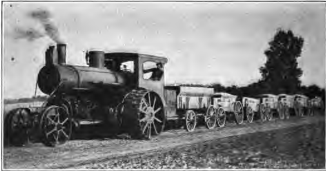
Fig. 251. An undermounted double-cylinder steam tractor.
