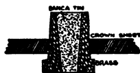
Fig. 244. A fusible plug, which is placed in the crown sheet as shown at F in Fig. 241.
