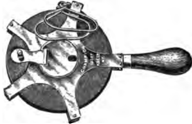
Fig. 3. A steel tape wound on a reel.
