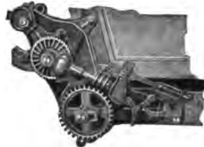
Fig. 185. One type of driving mechanism to the apron.
