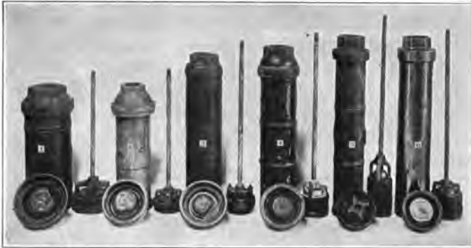
Fig. 303. Some common types of pump cylinders. 1 is of plain cast iron, 2 is galvanized, 3 is porcelain lined, 4 and 5 are brass lined, and 6 is an all-brass cylinder.
