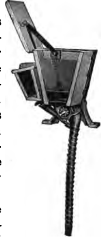
Fig. 141. A section of the seed box of a drill showing location of the grass seed box and a steel ribbon tube.
