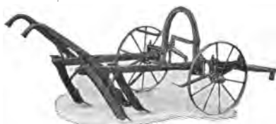
Fig. 147. A tongueless walking cultivator with wooden gangs.
