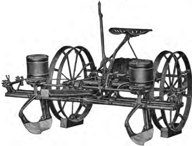
Fig. 142. A modern corn planter with long shoe furrow-openers, variable drop, and open wheels.
