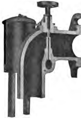
Fig. 219. A gasoline carburetor. The gasoline is vaporized by the air as it is drawn past the nozzle.
