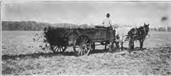
Fig. 183. A modern manure spreader at work.
