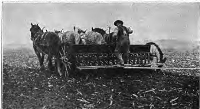
Fig. 137. A standard single-disk drill at work. This machine has 18 furrow-openers spaced 7 inches apart.
