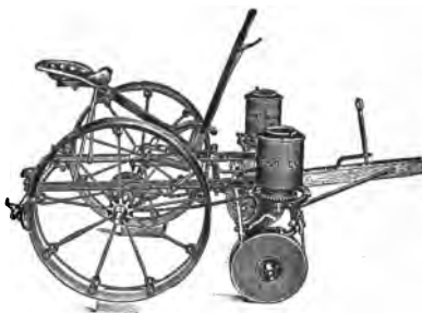
Fig. 145. A corn planter with disk furrow-openers.
