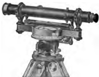
Fig. 35. A level known as a Wye level with horizontal circle and compass.
