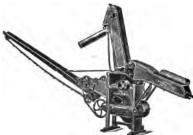
Fig. 189. A small two-hoe picker-wheel sheller equipped with self-feeder, cob carrier, and elevator.
