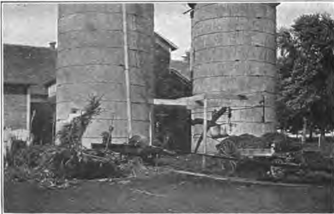
Fig. 174. An ensilage cutter of the radial-knife type equipped with blower at work.
