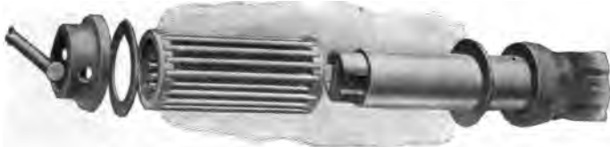
Fig. 103. A roller bearing for wagons. The hub of the wheel fits over the rollers shown.
