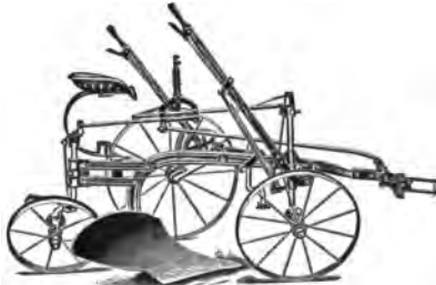
Fig. 112. A frameless and tongueless sulky plow guided by the hitch.
