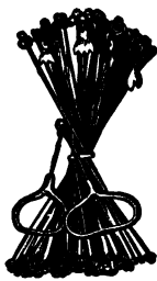
Fig. 1. The Gunter's chain, folded.
