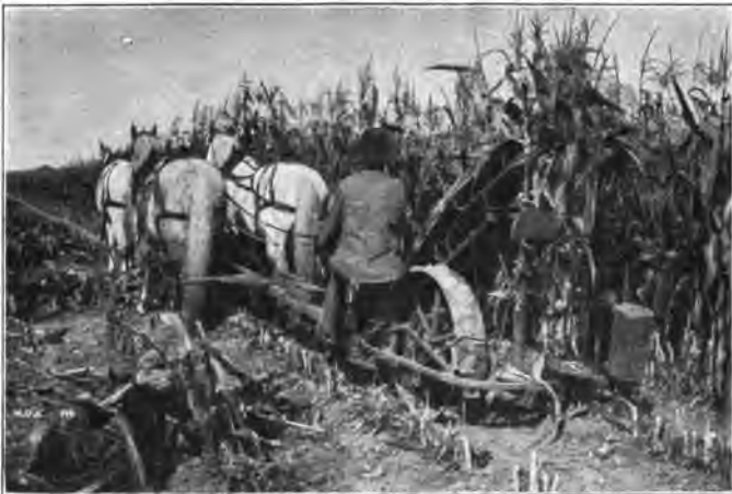
Fig. 157. A corn harvester of the vertical type at work.
