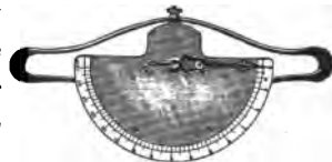
Fig. 198. A direct-reading traction dynamometer.
