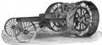
Fig. 239. The truck for a gas tractor, showing frame, gearing, and steering and driving wheels.
