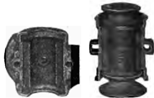
Fig. 128. A good form of bearing for disk harrows.
