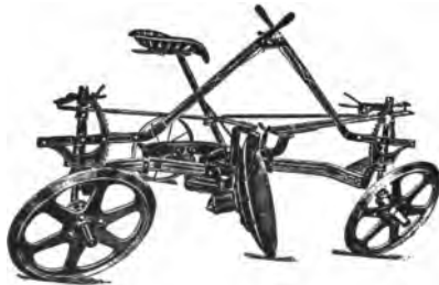
FIG. 117. A reversible disk plow. This plow is made to turn a right or left furrow by swinging the hitch from one end to the other.
