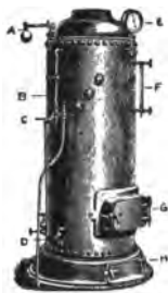
Fig. 240. A vertical boiler, showing A, safety valve; B, try cocks; C, injector; D, hand hole; E, pressure gauge; F, gauge glass; G, fire door; H, ash door.
