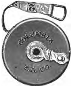
Fig. 2. A metallic tape. This tape has brass or copper wires woven into it lengthwise.
